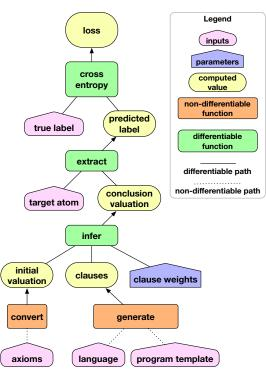
Figure 1: The  $\partial$ ILP Architecture.
