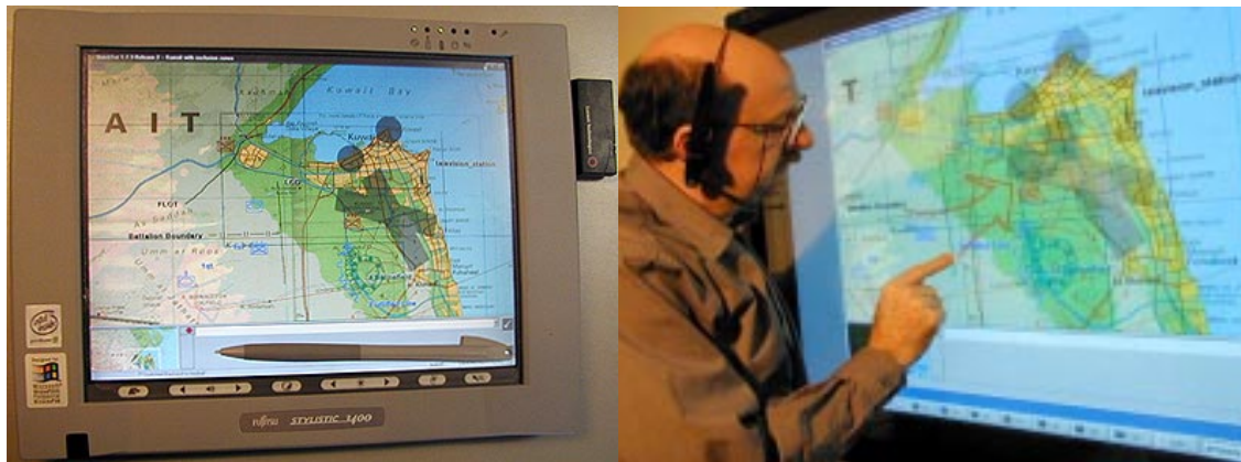
Figure 1: Left: QuickSet operating on a handheld PC; Right: Collaborating QuickSet operating on a 50" plasma display with touch overlay. User is speaking through a wireless microphone while drawing.
