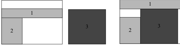
(a) Usable space is fragmented, item 3 cannot be packed (b) Item 1 is pushed upwards to make room for item 3
