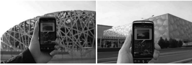
Figure 1: The developed mobile visual landmark search system, which embeds the compact visual descriptor extraction in HTC Desire G7 mobile phone, testing in typical areas like Beijing, New York, and Barcelona, etc.
