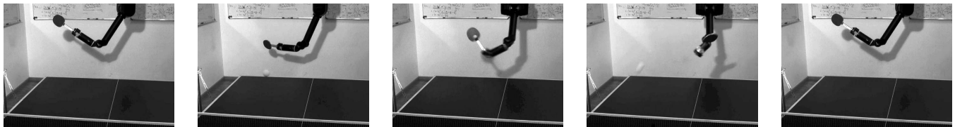
(a) The robot is in the rest posture. (b) The arm swings back. (c) The arm strikes the ball. (d) The arm follows through and decelerates. (e) The arm returns to the rest posture.
