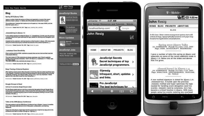
Figure 7: Flexible tree matching can be used to retarget Web pages designed for the desktop to mobile devices. Left : the original Web page. Right : the page automatically retargeted to two different mobile layouts.
