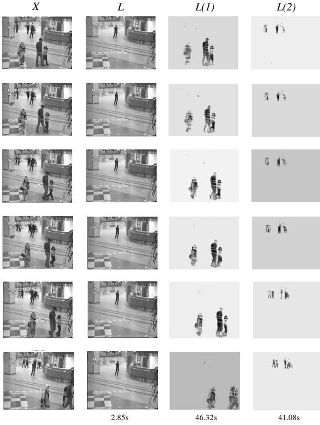
Figure 1: Background modeling and object flow tracking results of a 50-frame surveillance video sequence from Hall dataset with resolution 144 \times 176 .
