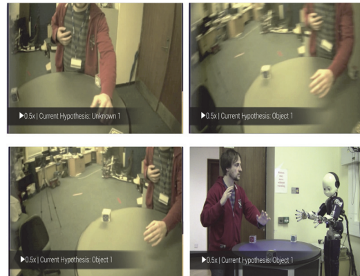
Figure 1: Experimental setup: iCub looking at target objects and arm movements (bottom right). The top-left image shows the iCub's gaze following the hand. In the top-right, hand movements of the human are anticipated by the iCub gaze. Finally, the bottom-left image shows gaze focused on the target object before the hand reaches it. These three images are grabbed from the iCub camera during an interaction trial.
