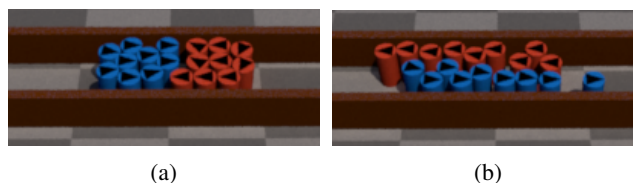
Figure 1: Two groups of 9 agents each move to the opposite side of a narrow corridor. a) ORCA agents get stuck in the middle. b) Agents using my coordination approach (C-Nav) coordinate their motion and reach their goals faster.
