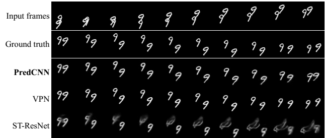
Figure 4: Visualization of predictions on Moving MNIST. We use 10 real frames as input and predict the next 10 frames recursively. We visualize the result of PredCNN using non-overlapping structure.
