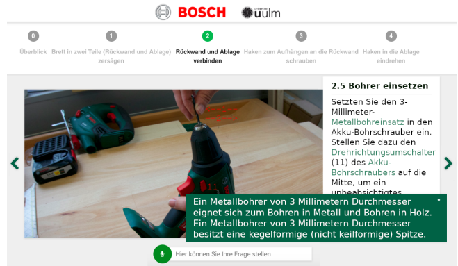
Figure 2: Instructions for inserting a metal drill bit, the green box contains the description of a metal drill bit requested by the user.
