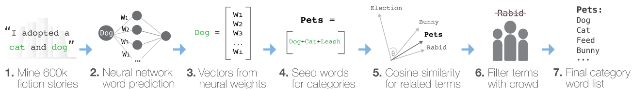
Figure 1: Empath learns word embeddings from 1.8 billion words of fiction, makes a vector space from these embeddings that measures the similarity between words, uses seed terms to define and discover new words for each of its categories, and finally filters its categories using crowds.
