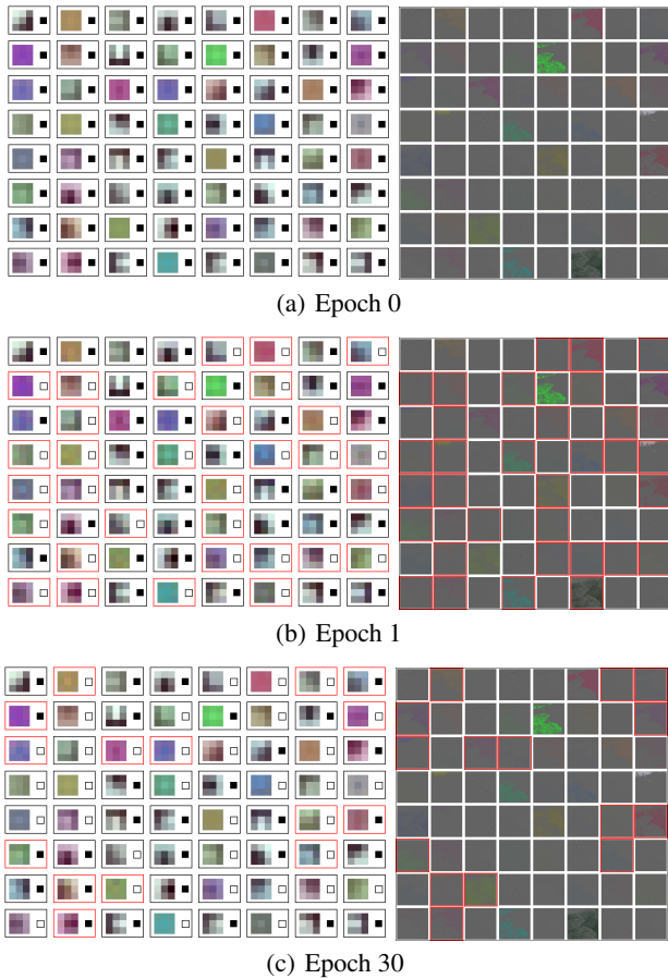
Figure 4: Dynamically update filters, masks and output feature maps on the first layer of VGG-16. Left: filters and masks, Right: output feature maps. In the left column, each rectangle contains filter and mask, in which the black one indicates the mask is unchanged, and the red one presents the filter and mask are updated. In addition, the mask is a smaller rectangle, in which ■ indicates the corresponding filter is salient, and □ is unsalient. In the right column, the feature maps changed correspondingly are shown in the red boxes.
