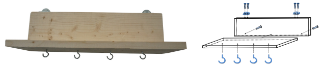
Figure 1: A real key rack and its conceptual drawing.
