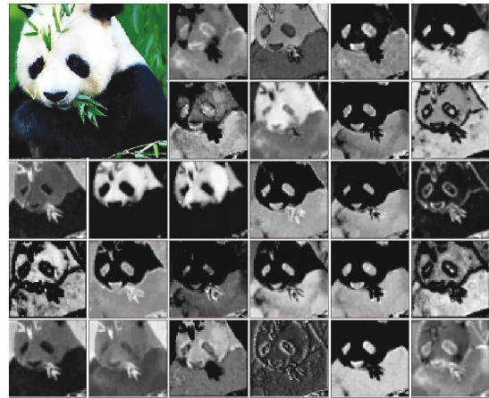
Figure 1: Visualization of input image (top-left) and some input feature maps of the second stage in ResNet-50. Many of them appear much pattern similarity. Therefore, some representative feature maps can be chosen to supplement intrinsic information, while the remaining redundant only need to complement tiny different details.
