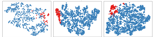
Figure 3: Visualization of representations on Celeb-DF(v2), FaceForensics++ and DFDC (from left to right). Red: Real, Blue: Fake.
