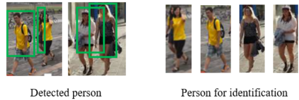
Figure 2: The detection-identification inconsistency problem. The detection model learns person proposal based on common person appearance using intersection-over-union (IoU) over certain threshold, which may result in less accurate bounding boxes compare to person for the identification task.
