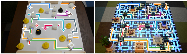
Figure 7: An OTIMAPP execution with 10 robots in an 8 \times 8 grid. Colored arrows represent an OTIMAPP solution.
