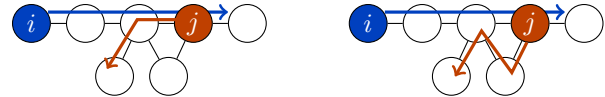
Figure 1: Example of OTIMAPP. A graph is depicted with black lines. Two agents ( i, j ) and their paths are colored. left : Both agents stop progression permanently due to mutual exclusion (i.e., no collision) if i moved two steps before j moves. right : As long as each agent follows a respective path, both agents eventually reach their last vertex; these paths constitute an OTIMAPP solution.
