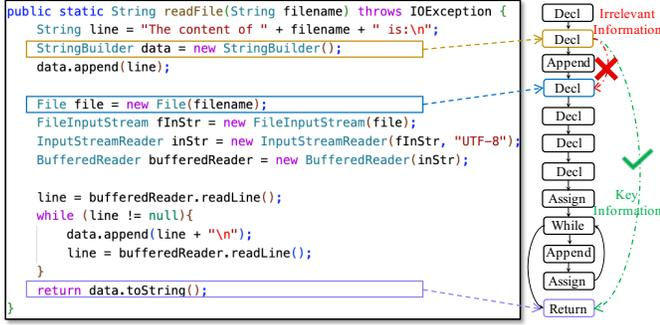
Figure 1: An example of the source code and the corresponding CFG. The declaration in the red box is the key information about the return value in the green box, while it takes entire eight steps to propagate it via the graph neural network.
