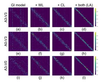
Figure 4: Attention weight map between different audio-visual sequences with LA method: row 1:  $(X_A^3, X_V^3)$ , row 2:  $(X_A^0, X_V^3)$ , row 3:  $(X_A^3, X_V^0)$ . The column 1-4 denotes GI model, GI + WL contrastive learning, GI + CL contrastive learning, GI + both (LA), respectively. The x-axis denotes visual frames in an utterance and y-axis denotes the audio frames in utterance, which is selected from LRS3 test set.
