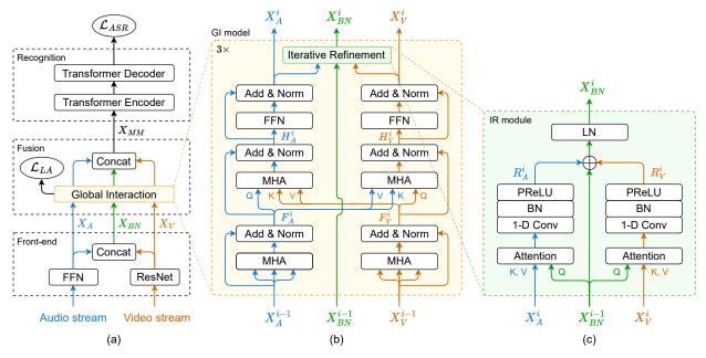
Figure 1: Block diagrams of proposed GILA: (a) Overall architecture, (b) Global Interaction (GI) model, (c) Iterative Refinement module. The  $\mathcal{L}_{ASR}$  denotes speech recognition loss, and  $\mathcal{L}_{LA}$  denotes local alignment loss.
