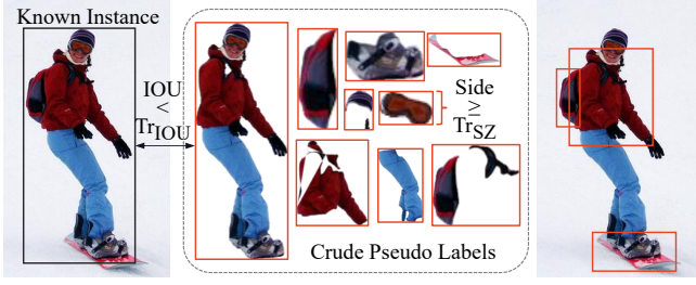
Figure 4: An illustration of pseudo-label refinement. We employ both IOU and the shortest side to filter the generated candidates. IOU is utilized for filtering annotations of known categories, while the shortest side is used for noise reduction.
