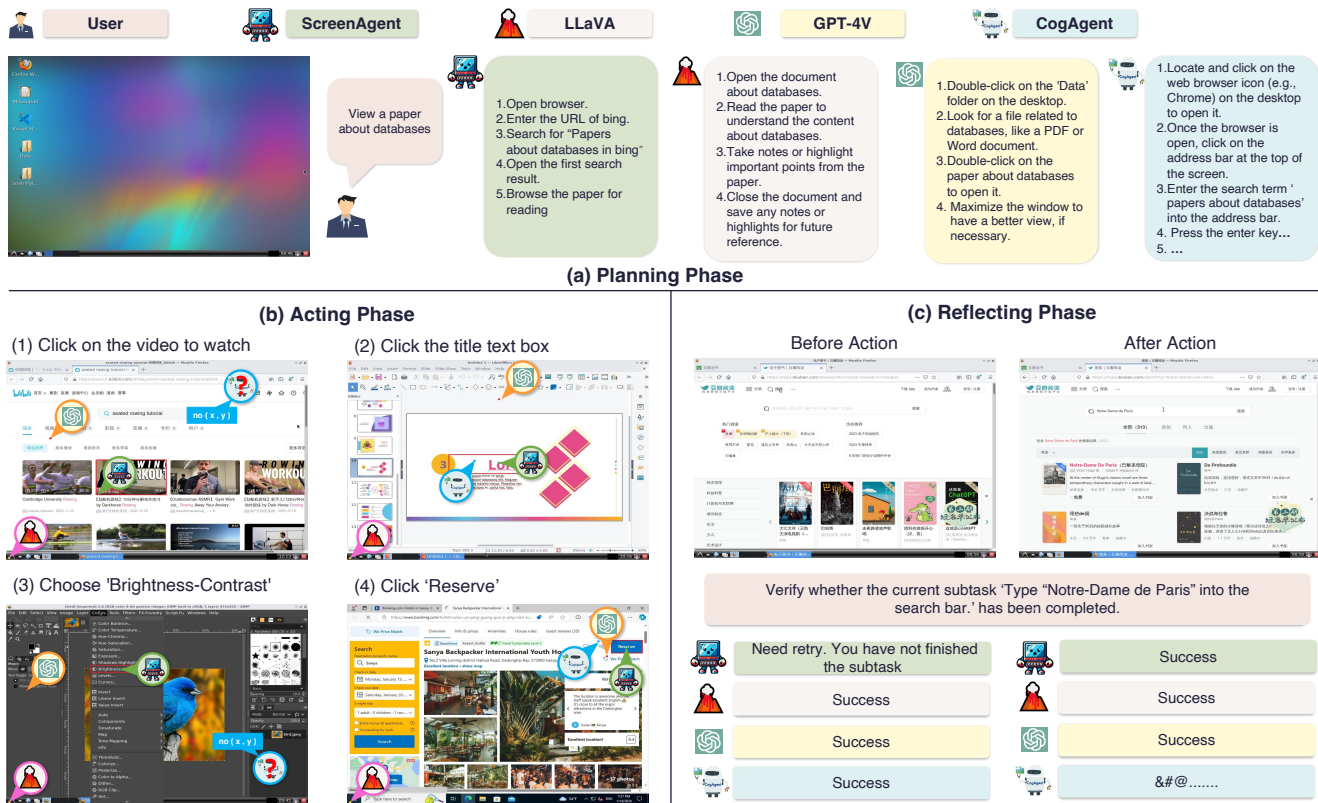
Figure 8: An example to show the execution results of multiple VLM agents among the planning, acting, and reflecting phases.
