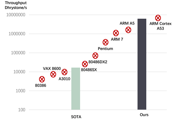
Figure 3: CPU performance comparison with the state-of-the-art. We compare the performance of the automated designed CPU designed by our method and the state-of-the-art. The red data points are human-designed commercial CPUs with similar performance. The result shows that our design is comparable to Arm Cortex A53 (2010s CPU), while the state-of-the-art automated design is only comparable to Intel 486 (1990s CPU).
