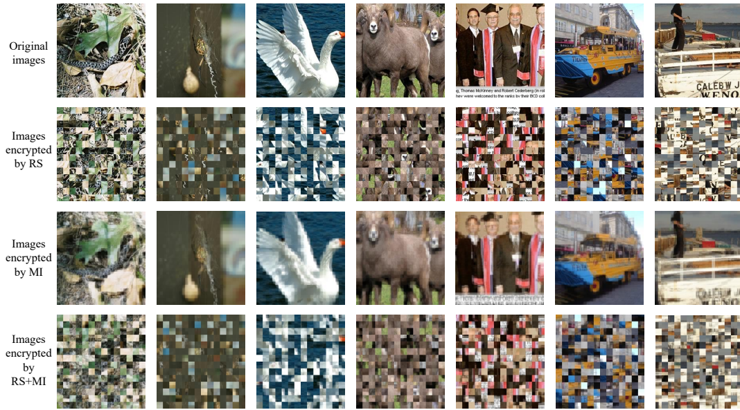
Figure 1: Illustration of images encrypted by RS, MI, and their combination. The visual contents of encrypted images are near-completely protected from recognizing by human eyes.
