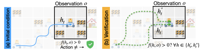
Figure 3: RNN-VERIFICATION for RL navigation: (a) The agent selects a safe action that avoids a collision. (b) The verification problem asks whether there exists a feasible history h (e.g., h'_t, h''_t ) such that the agent selects an undesired action, i.e., f(h, o) \leq 0 .
