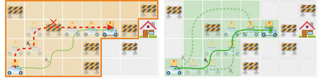
Figure 1: (Left) Interval-based verification over-approximates the hidden state space, admitting infeasible histories. (Right) RNN-PROVE assesses policies over probabilistically feasible histories, yielding more precise and informative certificates.
