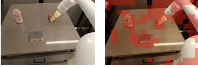
Figure 4: Left: input observation. Right: visualization of token-level importance predicted by the action-conditioned router, highlighting regions relevant to the current manipulation stage while suppressing distractors. The highlighted regions adapt with the action context, focusing computation on interaction-critical areas.
