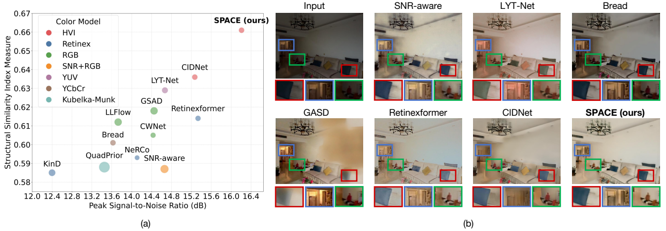
Figure 4: Comparison with advanced methods on the LAMP-Real dataset. (a) Performance Trade-off: Scatter plot of PSNR versus SSIM, where bubble color denotes the utilized color space and bubble size corresponds to the model parameter count. SPACE achieves the state-of-the-art balance. (b) Qualitative Evaluation: Visual comparison on a representative scene. Zoomed-in patches (red, blue, and green boxes) highlight SPACE's superior ability to restore sharp structural edges and suppress noise artifacts.
