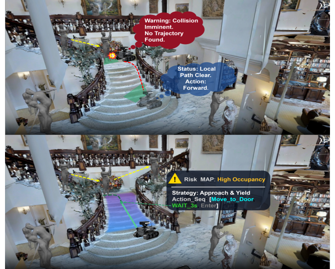
Figure 1: Navigation behaviours in a narrow corridor. (top) Reactive baseline: the agent relies only on a local cost map, blindly enters the narrow passage and gets stuck in a deadlock with an oncoming pedestrian. (down) AHead-VLN: the agent anticipates future crowd risk, chooses to wait at the entrance, and then proceeds, thus avoiding the deadlock.
