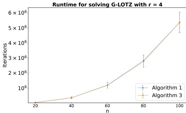
Figure 3: The mean (with standard deviations) number of iterations of Algorithms 1 and 3 for solving G-LOTZ with n \in \{20, 40, 60, 80, 100\} and r = 4 in 100 independent runs.
