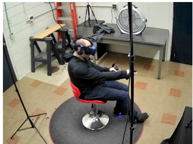
Figure 2: Participants were seated in a swivel chair with an HTC Vive headset. Shoe interfaces (Cybershoes) were strapped over their shoes allowing them to move through the simulation by making a walk motion. Valve Index controllers were strapped to hands for hand movements and shooting.
